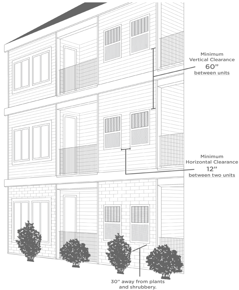
Fig 4: Recommended external clearances
